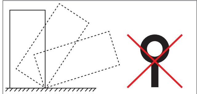
**Warning:** The top cover fixing bolts may NEVER be replaced with lifting eye bolts.
