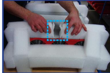
**Step 3.** Pull on one side of the foam to free the one side of the Flexa hand grip from the foam.
