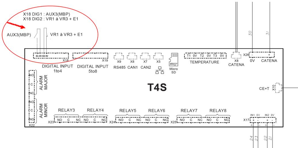
Aux 3 (from the by pass switch) : Provides an input to the controller indicating that the MBP is engaged
