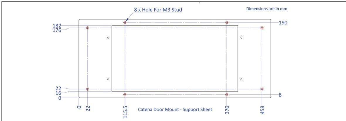
**Step 2.** Assemble the Door mount catena with the Catena support sheet using 4 x M3 studs.
