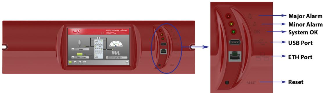
Remark: Reset will only reset the Catena, not the T4S and will have no effect on the system.
