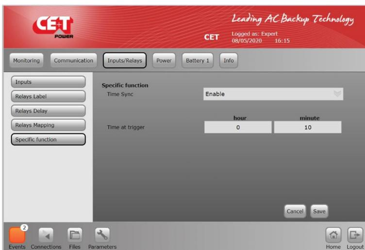
**Specific function** that can be used to synchronized time of T4S controller through an impulse on “digital input 08”.
