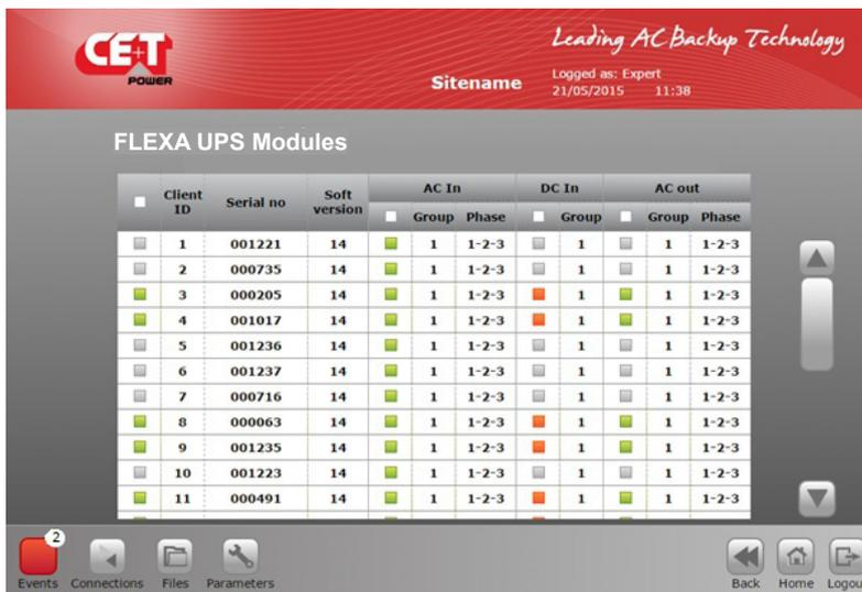
Table indicates the number of modules installed, ID, Serial number, Software version, AC IN, DC IN and AC Out details.
