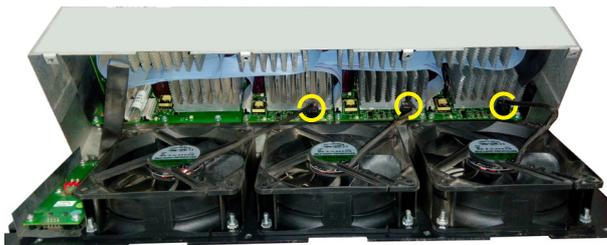
*Figure 3: Disconnect the fan wires*
