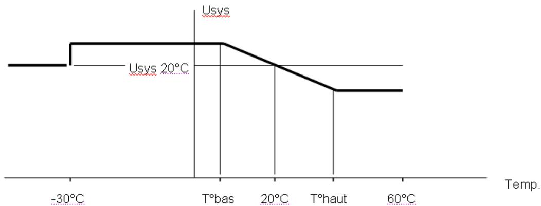
The MODE 2, charging voltage is adapted (provided it is enabled in the configuration) according the temperature. Using the charging curve below.
