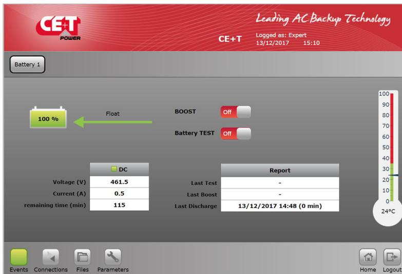
Battery x (x = 1 or 2) provide info on batteries status. The maximum DC group is two.
