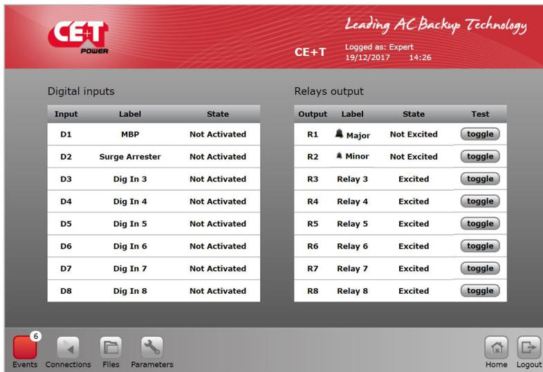
Present the output relay mapping with possibility to test each relay with the “toggle” button. Click and check relay changing status with an ohmeter.
