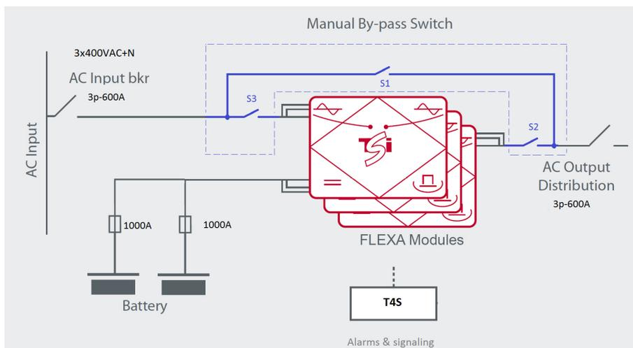
NORMAL mode or OFF: S1 is open, S2 and S3 are closed
