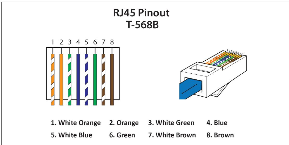
*Note: The colour of wires is irrelevant and may vary, but make sure the position of wires is exactly crimped.*
