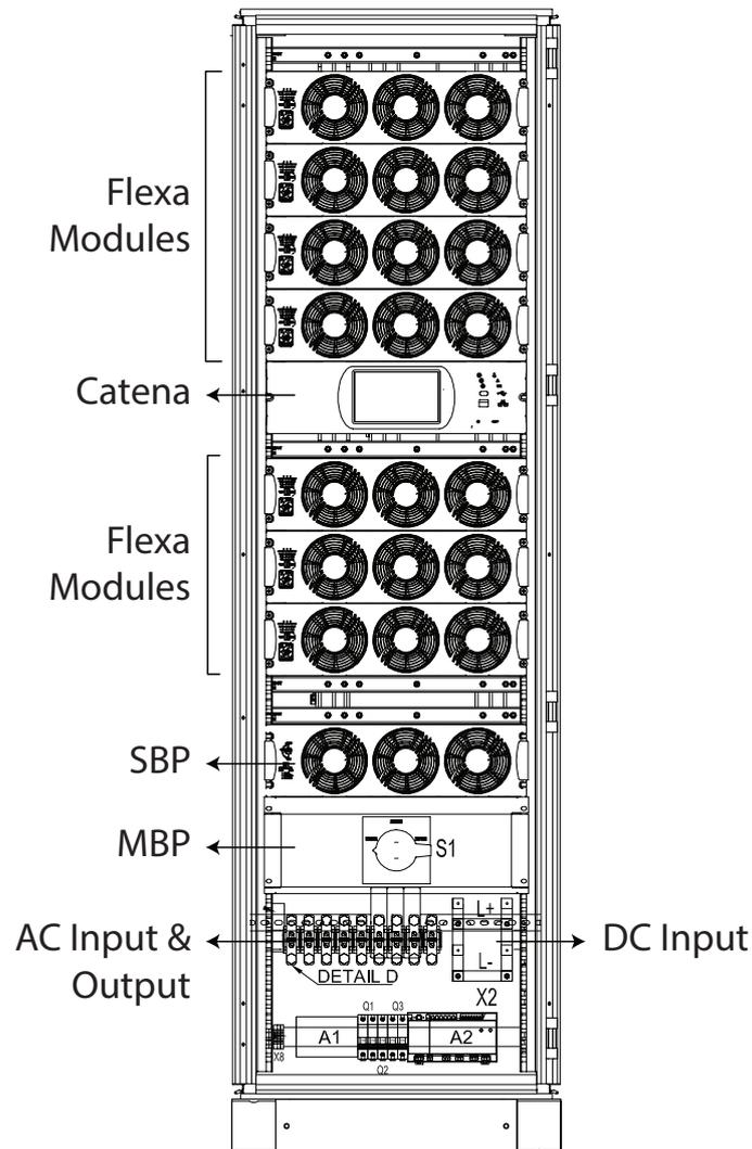
*Note: The above drawing is for general reference. Refer to the technical drawings received along with your cabinet for the exact arrangement.*
