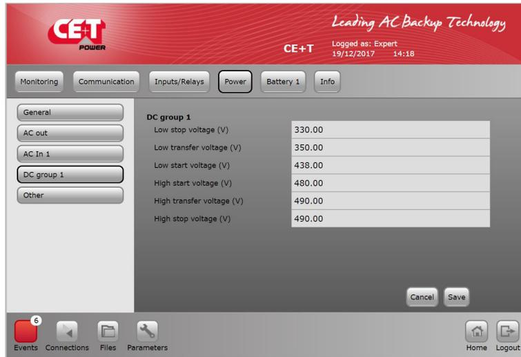
To configure DC input 1 Parameter. Low and High define voltage to configure boundaries min and max from where Flexa will STOP to preserve battery from deep discharge.
