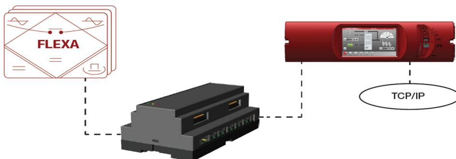
*Remark: Catena acts as a switch on the network. Both T4S & Catena need IP address as they are both connected to the network. See section 10.4.2, page 52 for tips on network configuration.*
