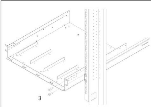
Fix cage nuts (4) in the mounting frame.
