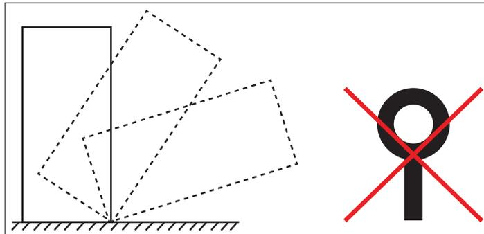
**Warning:** The top cover fixing bolts must NEVER be replaced with lifting eye bolts.
